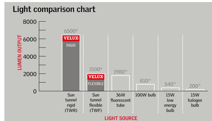
Light transmittance of VELUX Sun Tunnels depends on parameters such as sky conditions (cloudy/sunny), direction of sunlight, orientation and length of Sun Tunnel. VELUX Sun Tunnels in this chart have been tested with a 1 metre shaft, on a 15° roof pitch in summer, at noon on a sunny day using a photometer. (TWR rigid tunnel emits 440 lumens when measured on a cloudy winter's day).
